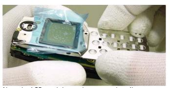
Now the LCD module can be removed easily.
