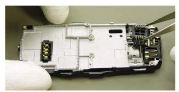
The SIM Connector can be removed with tweezers.
