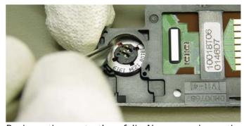
Replace the protection foil. Now you have the separated plastic frame of the LCD unit. You can now slightly push out the speaker with your fingers or tweezers.
