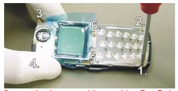
Remove the six screws with screwdriver Torx T6 in the shown order. When assembling the reverse order has to be taken with torque of 17Ncm.
