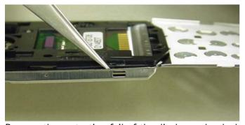
Remove the protection foil of the display and unlock the snaps on both sides of the display frame.
