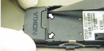
The Antenna is fixed with four snaps. It is enough, if you release with tweezers the two snaps at the battery side.
