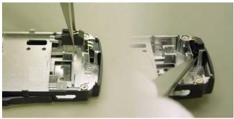
The Vibra Motor with its rubber case is squeezed into the B-Cover like the Microphone. Do not grab the spring connectors, because they may be damaged when pulling the microphone. To change the Microphone, push it up carefully with tweezers.
