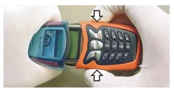
To open the unit the A-Shell has to be removed first. Press the grip markings on both sides of the B-Shell and pull the A-Shell apart from the B-Shell.
