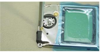
It is also possible to change the speaker, if needed. Therefore you have to unscrew these two screws. Remember to use torque of 8 Ncm when tightening the speaker screws.
